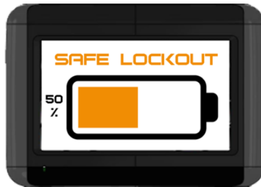
Figure 29: BDI Screen displaying ORANGE and SAFE LOCKOUT.
