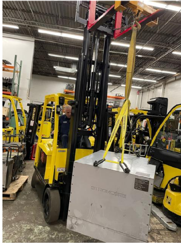
Figure 17: Image of battery lifted by 1 st forklift. Lifting straps are not twisted or pulling on any obstruction.
