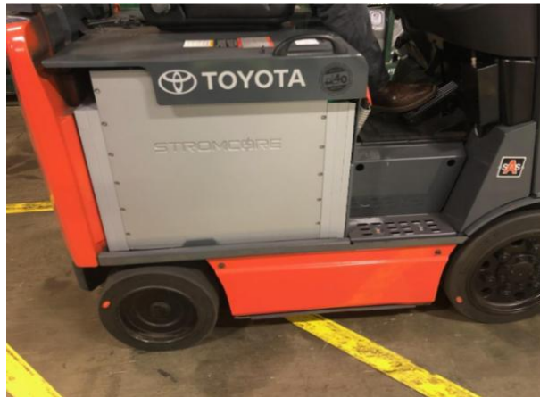
Figure 19: Example photo of battery tightly secured in the truck's compartment.
