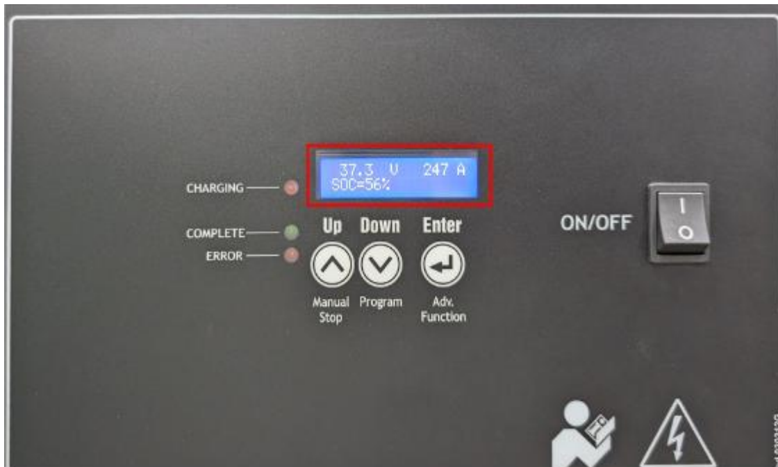
Figure 17: Photo reference of display screen showing charging parameters, indicating the charger is securely connected to the battery and is charging the battery.
