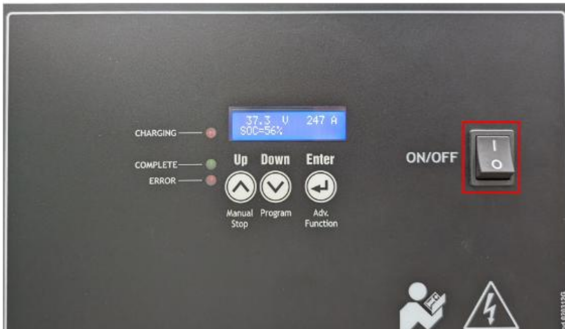
Figure 14: Charger switch is ON when “I” is pressed down.
