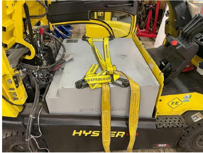
Figure 18: Image of sit-down truck with Stromcore Battery installed. Ports are facing towards the back of the truck.
