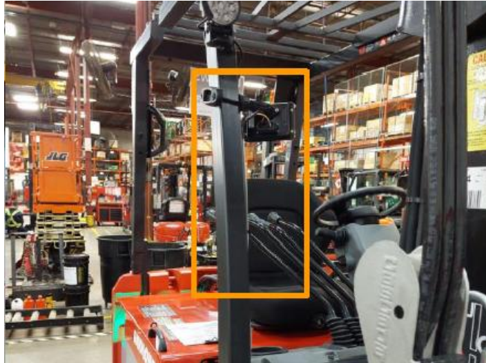
Figure 22: Image of BDI screen secured within the truck's compartment without any cables or harnesses at risk of being pulled, pinched, crushed, or damaged.
