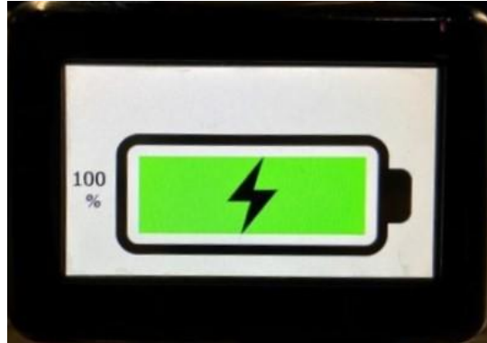
Figure 27: BDI screen displaying GREEN and Lightning Bolt.
